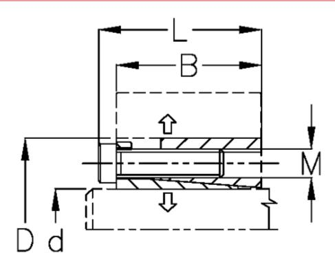
$\begin{array}{lll} \text{B mm} & = 101.0 \\ \text{d H8 mm} & = 340 \\ \text{D mm} & = 425 \\ \text{Fit tolerance} & = \text{Aksel h8, Nav H8} \\ \text{F kN torque} & = 1899 \\ \text{L mm} & = 121 \\ \text{M mm} & = \text{M20} \\ \text{P N/mm2 surface pressure on shaft/hub} = 168 \end{array}$
